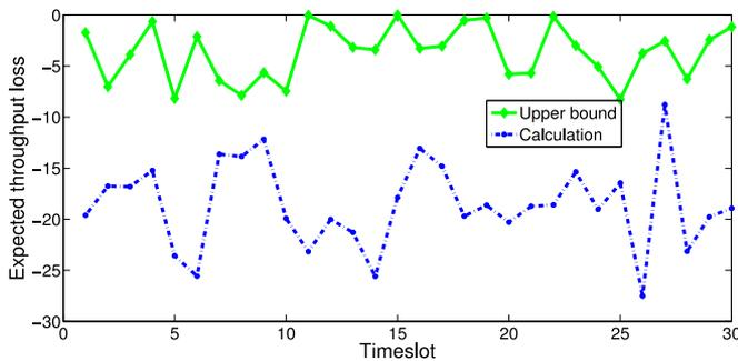
Fig. 8. Comparison of the calculated throughput loss per time slot for MTM with the upper bound of (17).
