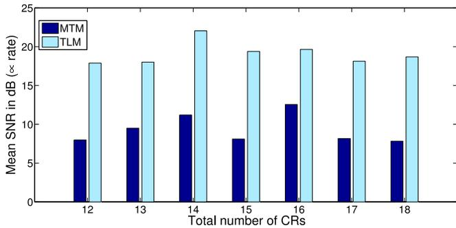
Fig. 7. Average SNR ( $\infty$  data rate) per time slot versus total number of CRs for TLM and MTM multiple access schemes.
