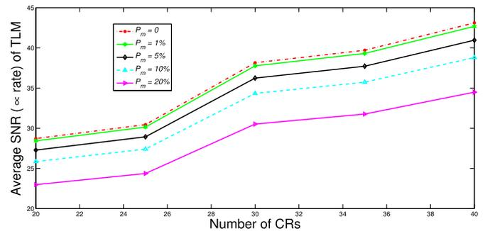
Fig. 10. Average SNR ( $\infty$  rate) for TLM versus the number of CRs for various probabilities of misdetection of PU ( $P_m$ )
