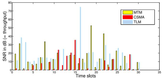
Fig. 4. SNR (proportional to rate) per time slot of the proposed TLM and MTM scheduling methods compared with that of CSMA.
