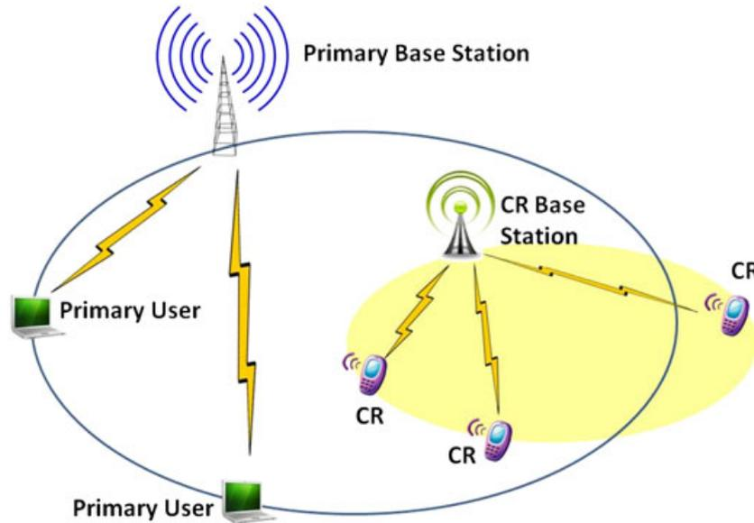
**Figure 1.** Primary providing unlicensed secondary cognitive radios with their spare spectral band.
