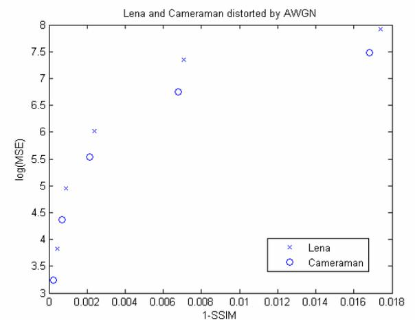
Figure 5- Simulation results for additive white Gaussian noise obtained through transmitting the whole approximation coefficients
