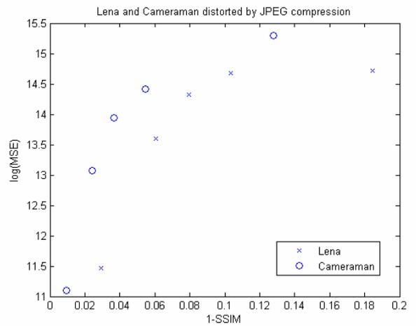
Figure 3- Simulation results for JPEG channel model obtained through transmitting the whole approximation coefficients
